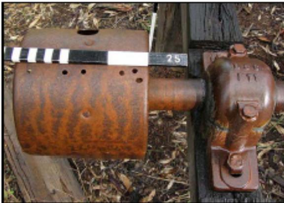
Plate 20 – Plank-saw belt cam and bearing
