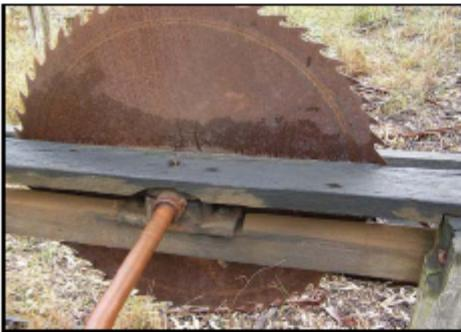
Plate 11 – Detail of the drive shaft and saw blade of the log-saw.
