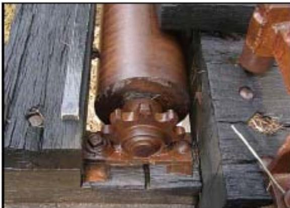
Plate 24 – Detail of western end of log-in roller (plank-saw).
