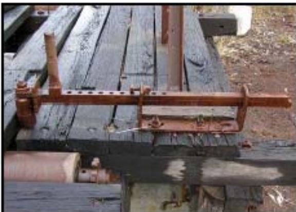
Plate 27 – Saw gauge in a closed (narrow plank) setting.
