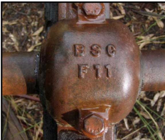
Plate 21 – Detail of the bearing housing.
