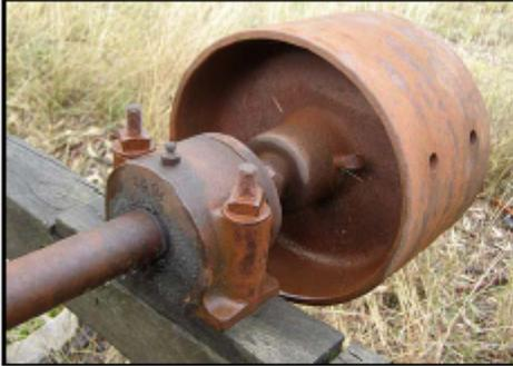
Plate 10 – Detail of the drive shaft and belt cam of the log-saw.
