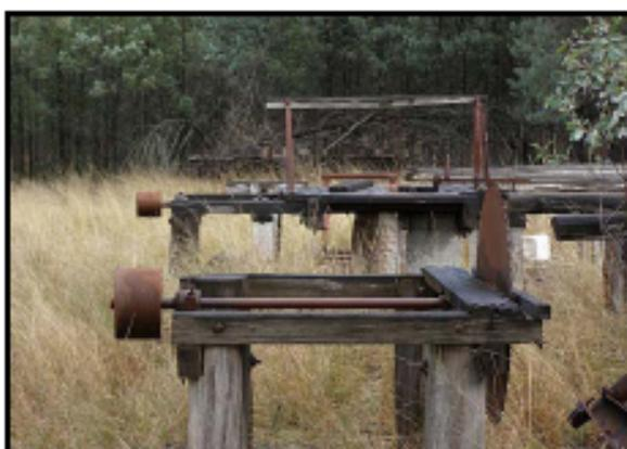
**Plate 6 – View showing the alignment of the belt cams.**
