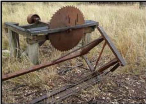
Plate 32 – View showing the length of railway-track rail attached to the base of the trolley to act as a counter-weight to that of the log.
