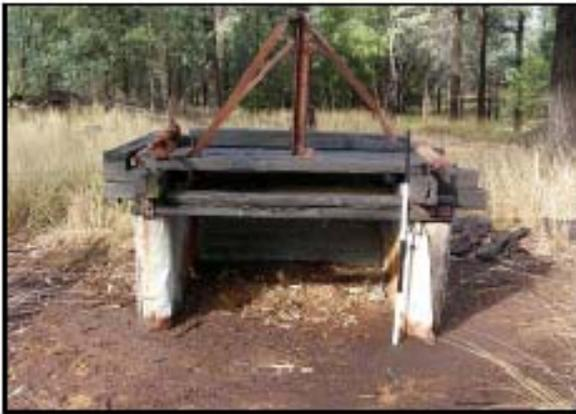
**Plate 29** – View of the plank-saw from the west, showing the sawdust chamber beneath the bench.
